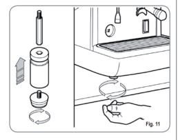
It is advisable to install a softener (1) and then a mesh filter (2) on the external part of the plumbing system, during preliminaries and after levelling the machine.
