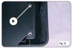
• Turn the pump registration screw, turning it clockwise to INCREASE and counter clock wise to DECREASE the pressure.
