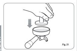
Press the coffee with the provided coffee presser, dust off any coffee residue from the rim of the filter (this way the rubber gasket will last longer).
