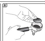
Insert the rubber disk into the filter-holder with its filter.
