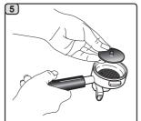
Insert the rubber disk into the filter-holder with its filter.
