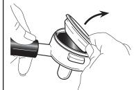
Remove the filters from the filter-holders.
