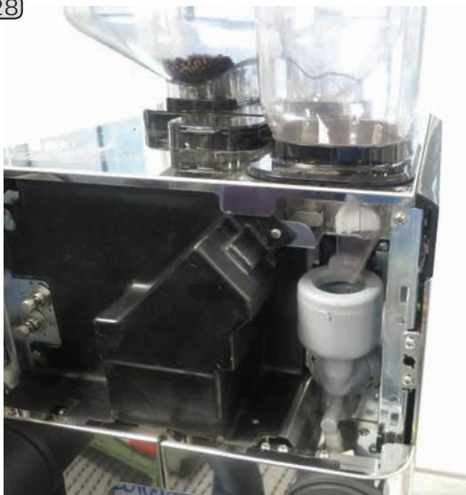
Re-assemble the other mixer parts according to disassembly rules.
