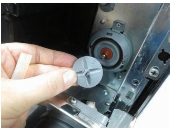
Put correctly the polarized wheel (the arrow must be directed to the plane part of the stainless steel motor shaft).
