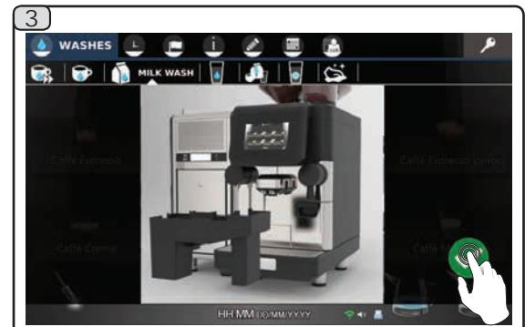
The steps for performing a milk wash are shown on the touch screen; at the end of each phase, press the icon
