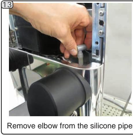
Remove elbow from the silicone pipe.
