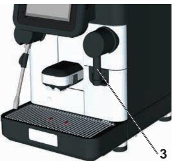
After the icon appears, 10 more coffee-based beverages can be dispensed, after which an animation will be seen on the touch screen to empty the drawer. Any additional dispensing is blocked and the grounds drawer must be emptied.
