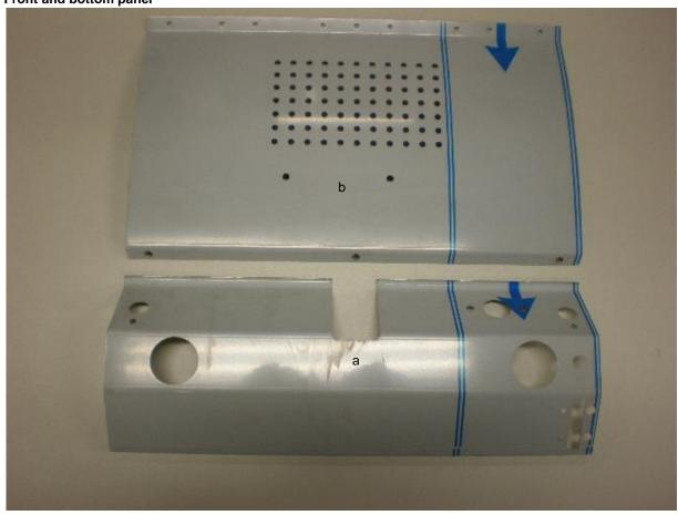
Panel-work has changed a few times since production of the Speedster started. Major changes for the front panel are to allow for the wider group neck and later to accommodate the shot-timer display. The bottom panel has gained perforations for better air-flow around the machines' electronics. Newer parts may or may not fit on older machines.
