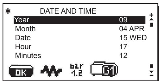
Use the "+" (30) and "-" (31) keys to move the cursor (black line) to the entry to be modified, then press the PRG (29) key. The cursor will turn into an arrow and it becomes possible to change the number for the selected entry by using the "+" (30) and "-" (31) keys.
