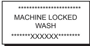
When the key corresponding to the wash requested in the message (key 26 or key 28), the wash cycle is activated and the machine is unblocked.
