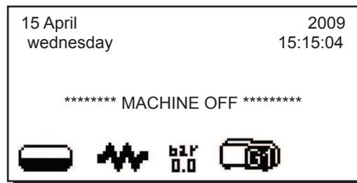
**N.B. When the machine is working in the automatic on/off function do not use the general switch (23) to switch off the machine. If this happens, the machine will not be able to switch on again automatically.**
