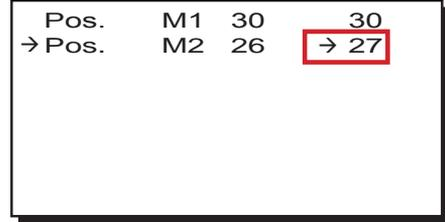
The setting for both grinders has a field range of ± 5 of the value set in the technical programming menu.
